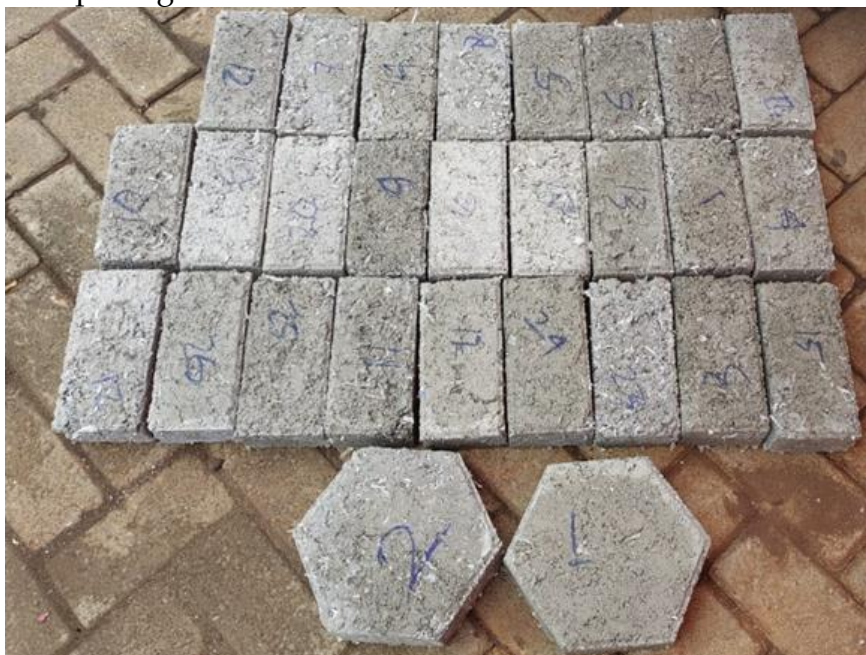
Figure 9. Final Result of Paving Block Mold using Plastic Waste Mixed Material
